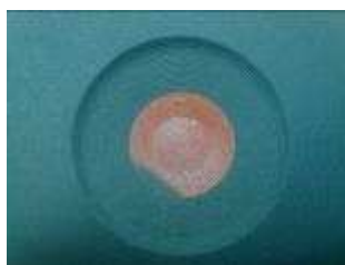
Picture 20: example of bad print on the edge of red dot
